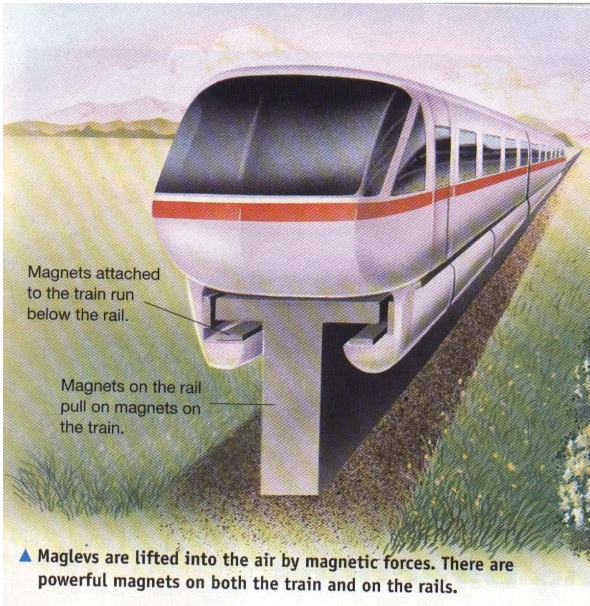
Magnets attached to the train run below the rail.
